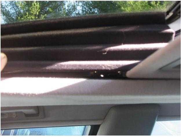
3) Push the bellows up out of the way and pull the 3 T20 bolts per side- the one way in the front and the one in the back are the hardest to get at (picture with bolts already out). Don't worry if you drop them during removal- they're easy to retrieve once you pull the sunroof panel. Once all 6 bolts are out, the sunroof just lifts out the top.
