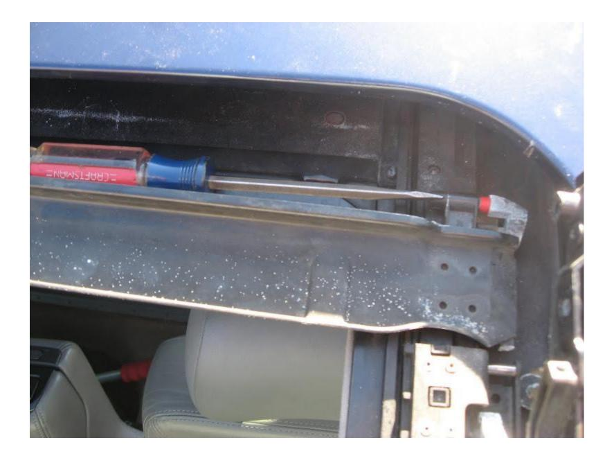
7) This is what the rain tray looks like out of the car. The strap attaches the rain tray to the sunshade so that it pulls forward automatically.
