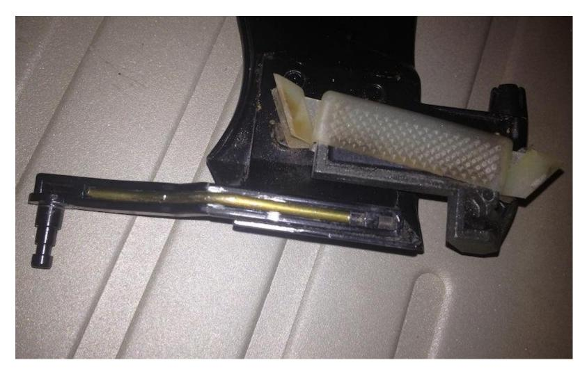
And now the epoxy is curing. The electrical tape is just precautionary to keep the arm from falling.
