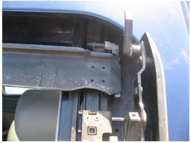
6) The rear mounts are harder to get at, and harder to get to release. What I've found works the best is using 2 screwdriversone inserted as shown to push the arm out of the mount, the other prying open the slots in the clip. Again, be gentle because the metal isn't very strong. The good news is you only have to release one side. Once the near side is out, push the rain tray away from you and it should just lift out. Make sure you get the nylon guide that sits in the track.
